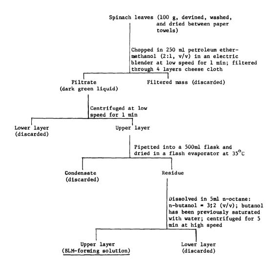
Fig. 1. Scheme for extraction and preparation of BLM-forming solution from spinach leaves.
